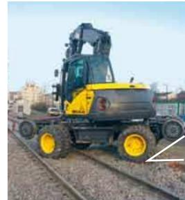
The minimum front and rear passage angle of 30° makes it easier to enter and leave the railway track or to pass over obstacles (embankments for example).
