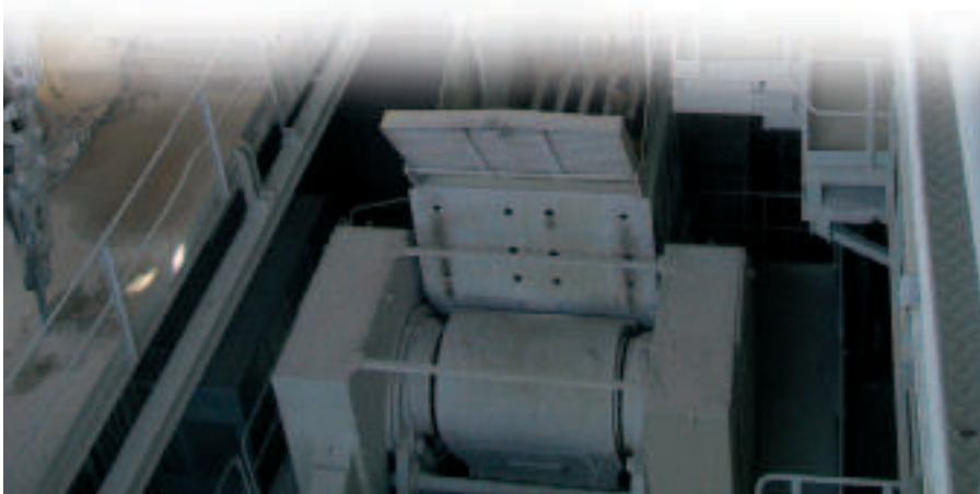
A C200 after replacement of a double toggle jaw crusher. Plant capacity was increased without having to modify the foundations.
