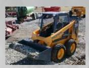
OFFSET LOAD-ARM ▲ design creates a wider operator's compartment, and an optional suspension seat adds even more comfort.
