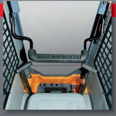
UNIQUE RESTRAINT BAR △ design ties into the Hydraloc<sup>™</sup> safety system, provides added protection and is fully adjustable for an ergonomic and safe operator's environment.
