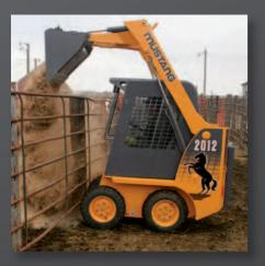
**MOVE MORE** A with a lift height of 2438 mm which makes loading and material handling in small spaces easy.
