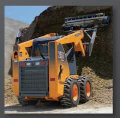
OPTIONAL POWER-A-TACH® A hydraulic attachment system allows the operator to change buckets and attachments without leaving the seat.
