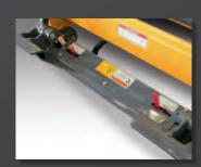
POWER-A-TACH® SYSTEM \_\_\_\_ optional on many models, this system allows users to quickly install and remove attachments, leaving the seat only to connect auxiliary hydraulics.
