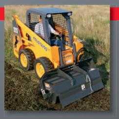
**MULTI-TASK** with a variety of attachments that can be powered by the auxiliary hydraulic system.
