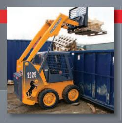
HIGH LIFT HEIGHTS ▲ of up to 2794 mm make material handling in small, confined spaces easy.
