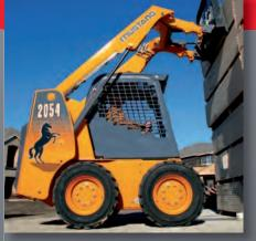
HIGH LIFT HEIGHTS ▲ of up to 2946 mm coupled with the compact machine design make material handling in small, confined spaces easy.
