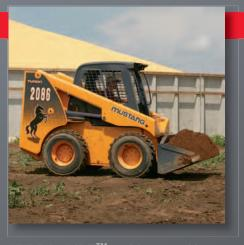
HYDRAGLIDE™ ▲ ride control is a standard feature with certain control configurations that allows the bucket to "float" in carry position, reducing the amount of material spillage.
