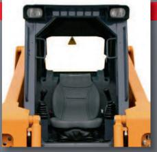
**ROOMY CABS \( \rightarrow\$** come standard with an adjustable suspension seat (optional on 2056 Series II), dome light, work lights, and choice of hand/ foot, dual hand or joystick controls.
