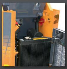
**EASY MAINTENANCE** A with the tiltable ROPS/FOPS and wide rear door provides access to service and maintenance points.
