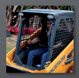
are available to fit the needs of any operator. Control configurations include: dual lever with foot controls, dual lever with hand controls, and T-bar with foot controls.
