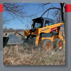
AUXILIARY HYDRAULIC ▲ system powers a variety of attachments.
