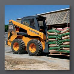
**HIGH START-UP TORQUE** for rapid acceleration with or without a load is made possible by maintenance-free, radial-piston drive motors.
