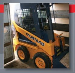
NARROW MACHINE WIDTH ▲ of only 914 mm with 5.70 x 12 chevron tire set, and 1118 mm with 8.50 x 12 HD flotation tire set allows the 2012 to gain access where other machines can't go.
