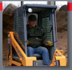
ALL-DAY COMFORT ▲ and protection in the operator-friendly ROPS/FOPS Level II-certified cab. A high-back, deluxe seat comes standard, a high-back suspension seat is optional.
