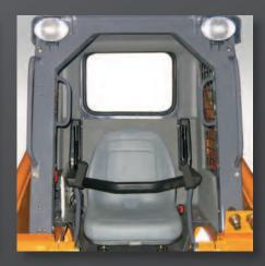
UNIQUE RESTRAINT BAR ♣ design is tied into the Hydraloc<sup>TM</sup> safety system, assuring operator safety by preventing engine start-up when the operator is not in the seat with the restraint bar in place.
