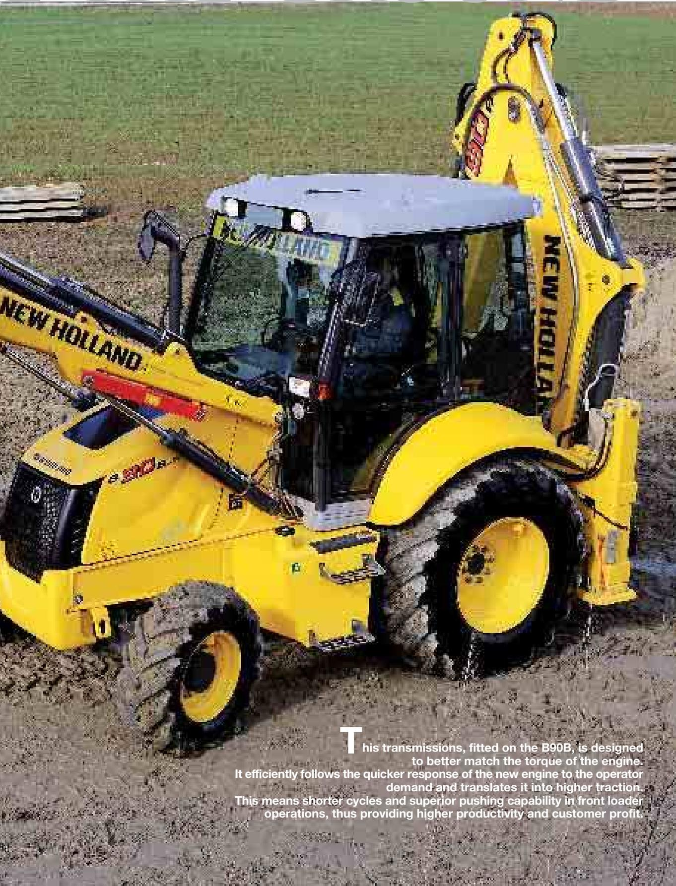
**T**his transmissions, fitted on the B90B, is designed to better match the torque of the engine. It efficiently follows the quicker response of the new engine to the operator demand and translates it into higher traction. This means shorter cycles and superior pushing capability in front loader operations, thus providing higher productivity and customer profit.
