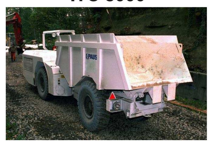
Tunnel articulated Dump Truck PAUS model ITC 8000 with all wheel drive and reverse seat
