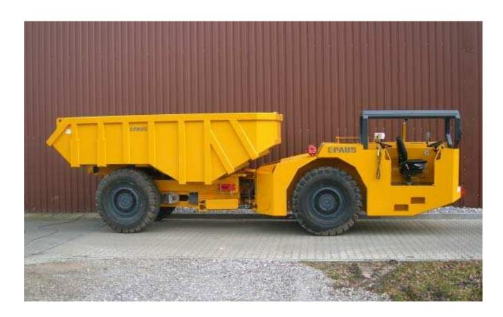
Tunnel articulated Dump Truck PAUS model ITC 12000 with all wheel drive and reverse seat
