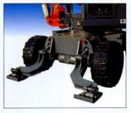
The EB 706P is equipped as standard with a sturdy blade controlled by two rams fitted with safety valves. In option, this can be replaced by two separately controlled stabilisers to which a removable blade can be added.
