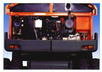
The back cover opens completely, giving excellent access to the engine and hydraulic pumps. All maintenance and checking points are conveniently located close to hand.
