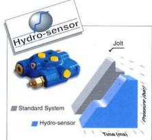
The hydrosensor valve (Pel-Job patent) on the slewing circuit damps the pressure peaks and hydraulic shocks common on starting and stopping on conventional circuits. The result: a progressive pressure increase, greater flexibility and precision and less stressed and therefore more reliable mechanical parts.
