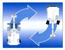
Pel-Job's Auto-Reverse system, available as an option, automatically reverses the steering direction when the excavator is facing the back. Thanks to this exclusive system, the wheels are always oriented in the direction of rotation of the steering wheel, for greater precision and safety in operation.
