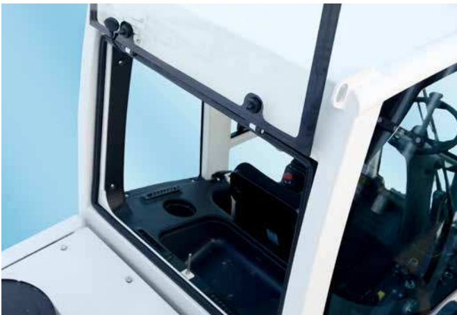
Opening rear window ensures convenient airing, can serve as an emergency exit in case of an accident and helps with maintenance and repairs.
