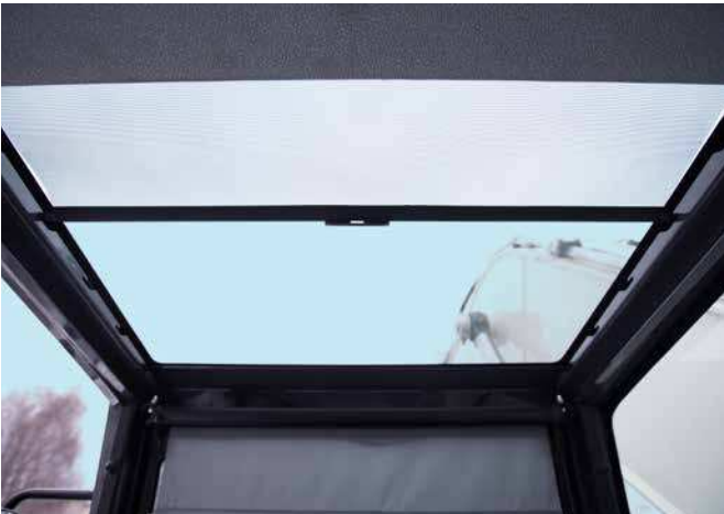
Adjustable roller blinds on the upper and front windows protect the operator from bright sunlight (standard).
