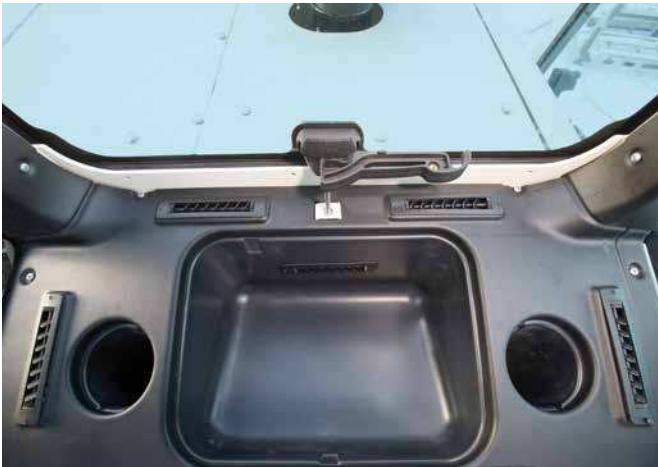
Slotted and rotating deflectors provide efficient window blowing and prevent windows from freezing and fogging.
