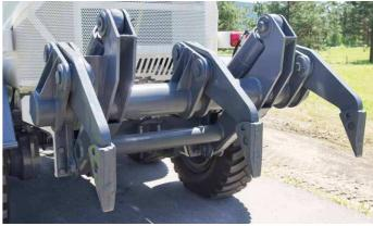
Rear ripper is used to loosen compacted or heavy soil and break road cover.
