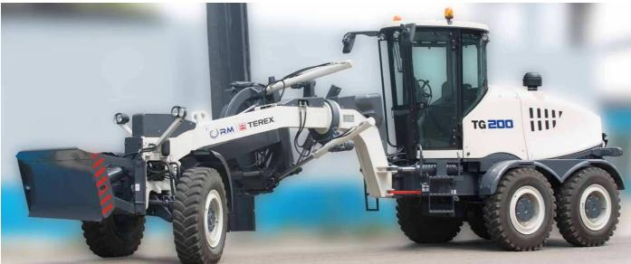
T-frame drawbar is designed to handle heavy loads. The moldboard hydraulic cylinders feature hydraulic locks fixing the moldboard positions for precise blading control.
