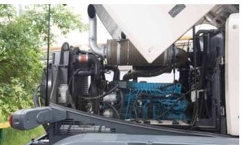
High-performance cooling is ensured by the state-of-theart Fan Drive system (electronically controlled hydrostatic fan drive). The processor receives signals from the radiator sensors and sets the required fan rotation speed.
