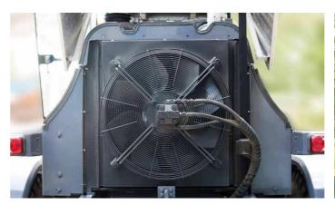
Integrated cooling system includes radiators for the engine, gearbox, and front axle hydraulic drive (if equipped).
