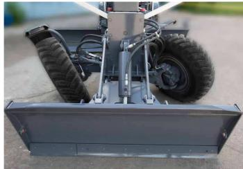
Front wheel lean feature helps when working slopes and compensates reaction forces on the moldboard in case of wide working angles.
