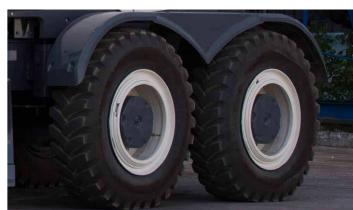
Rear bogie features robust fenders protecting the cab and hood from dirt which can be used as additional platform to carry out maintenance.
