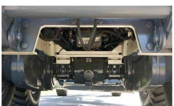
NAF tandem bogie paired with ZF automatic transmission delivers high drive wheel torque and traction in various operating conditions.
