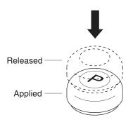
**NOTE:** When pressing the parking brake switch during machine running, the brake is activated and the engine is stopped at the same time. When starting the engine again, shift the F-N-R lever back to the neutral position, set engine speed to idle, activate the parking brake switch, and then start the engine.
