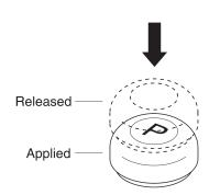
**NOTE:** When pressing the parking brake switch during machine running, the brake is activated and the engine is stopped at the same time. When starting the engine again, shift the F-N-R lever back to the neutral position, set engine speed to idle, activate the parking brake switch, and then start the engine.
