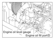
**NOTE:** When checking the amount of oils after running the engine, please check at least 15 minutes after the engine is stopped. If the machine is inclined, please move it to the flat ground before start checking it.
