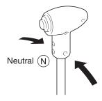
NOTE: When the F-N-R lever is not in the neutral (middle) position, or the parking brake has been released, the interlocking system goes into operation and the engine will not turn on. Be sure to confirm that the F-N-R lever is in the neutral (middle) position, and that the parking brake is engaged before starting the engine.
