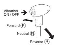
Provided at the knob of the lever is the vibration switch for turning on or off the vibration.
