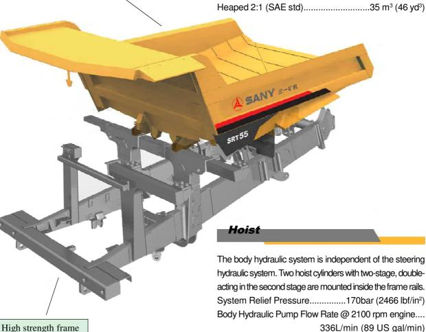
The body hydraulic system is independent of the steering hydraulic system. Two hoist cylinders with two-stage, doubleacting in the second stage are mounted inside the frame rails. System Relief Pressure......170bar (2466 lbf/in²) Body Hydraulic Pump Flow Rate @ 2100 rpm engine....
