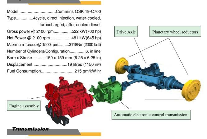
Allison M6610AR automatic electronic control transmission with Soft Shift feature. Integral TC 682 torque converter, hydraulic retarder and planetary gearing are mounted in the middle of the frame. Six speeds forward, two reverse. Automatic lock-up in all speed ranges. Hydraulic retarder. Body-up shift limiter.
