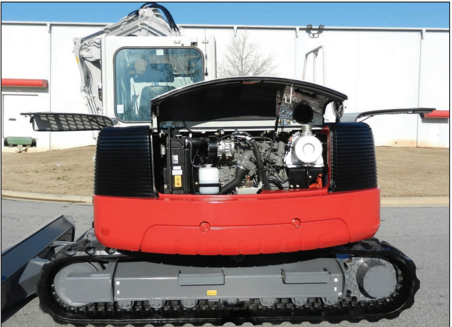
Large lockable service hood provide vandalism protection and outstanding maintenance access.
