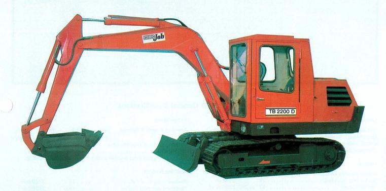
The TB2200 D, equipped with the quiet Isuzu Engine, C-240-P, provides extra power and superior digging depth, while being compact and economical in fuel consumption.
