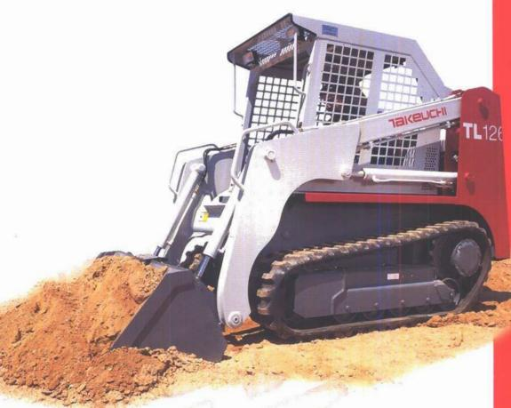
Rubber tracks combine the capabilities of a track loader with the versatility of operation on improved surfaces
