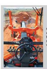
Good and wide visibility offers clear view of the mold board heel. The elevated operators seat helps in good rear visibility.
