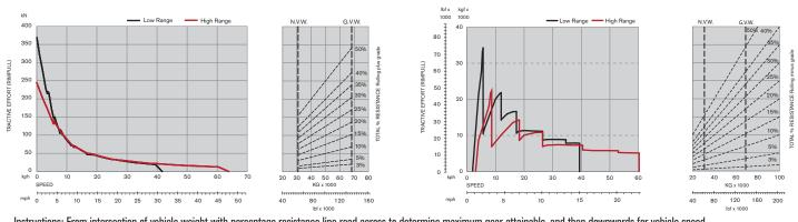
Instructions: From intersection of vehicle weight with percentage resistance line read across to determine maximum gear attainable, and then downwards for vehicle speed.
