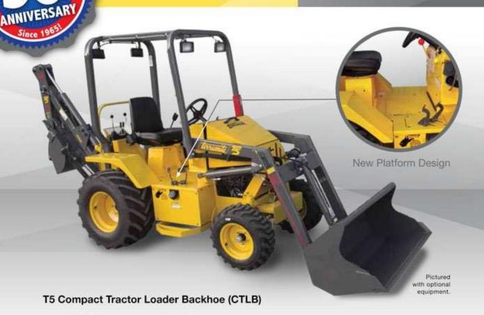
Terramite's T5 is compact enough to fit in many areas inaccessible to larger machines. It is a rugged machine and has the power to tackle many of the "big machine jobs", such as septic tank installations, water, sewer and gas lines, landscaping, spreading or loading.
