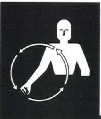
Fig. 8 START THE ENGINE Simulate cranking the vehicle by moving arm in a circular motion at waist level.
