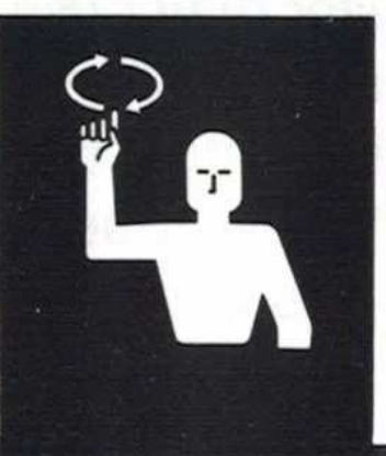
Fig. 11 RAISE EQUIPMENT Make circular motion with either hand at head level.
