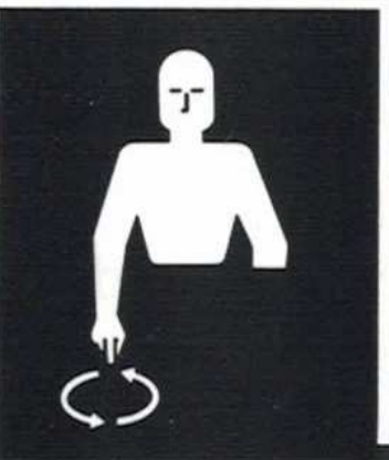
Fig. 10 LOWER EQUIPMENT Make circular motion with either hand pointing to the ground.
