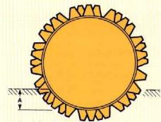
The method of calculating the ground pressure of a compactor in this case involves deducing the projected wheel drum area against the ground at various depths of penetration into the surface and relating the result to the axle loading of that wheel.
