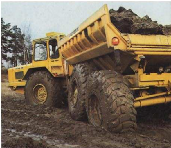
The bogie driving axle, designed for rugged off-road haulage, is provided with hub reductions and a differential lock.
