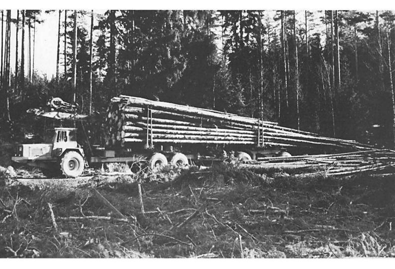
VOLVO BM 860 TC tree length hauler. Trailer with turntable ensures agile manoeuvrability. Accommodates logs up to 30 m in length.
