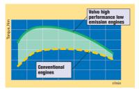
Volvo high-performance low-emission engines have considerably higher torque at low engine speeds than conventional engines. Maximum torque at only 900–1200 rpm means more strength and acceleration. The engines meet all current exhaust emission requirements.
