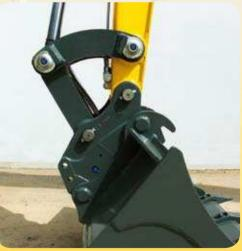
The innovative hydraulic EASY LOCK quick-hitch system is optimally suited to the kinematics of Wacker Neuson compact excavators and makes a decisive contribution to work process improvement. Just drive up, hook up and lock automatically. Its low headway means that the bucket displacement angle remains unaffected. Workflow improvement is guaranteed.
