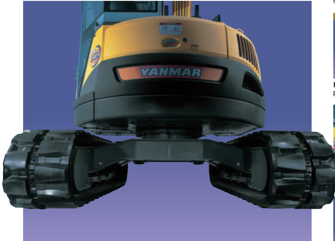
Large opening rear hood for easier maintenance.
