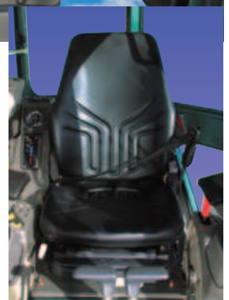
Reclining and suspension seat with seat belt.
