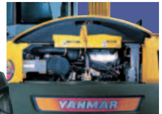
Large opening rear hood for easier maintenance.
