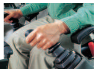
Joystick pilot controls and arm rests are convenient to use and reduce operator fatigue.
