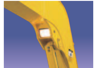
Integrated boom-light is protected from damage.
