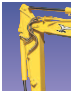
To enable the use of additional hydraulic attachments, PTO is piped to the end of the arm.
