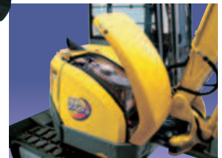
Battery, fuel and hydraulic oil can be checked more conveniently.
