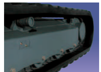
Angled crawler frame reduces unwanted build up of foreign matter.
